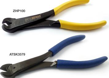
These tools are designed to cut away swaged or threaded collars from fasteners so the fastener pin can be easily removed. They are ideal for removing Hi-Shear<sup>®</sup> rivets.
